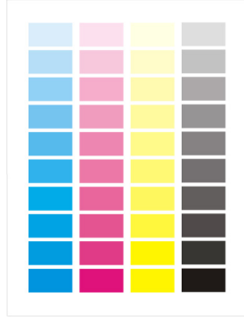
Figure 4. Test form with known CMYK image square areas.
