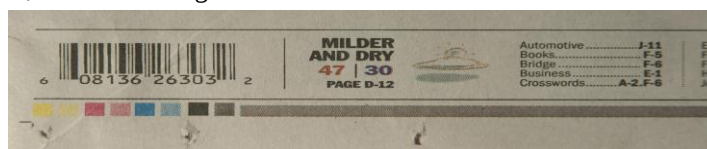
Figure 3. Solids and tints printed for process control.
