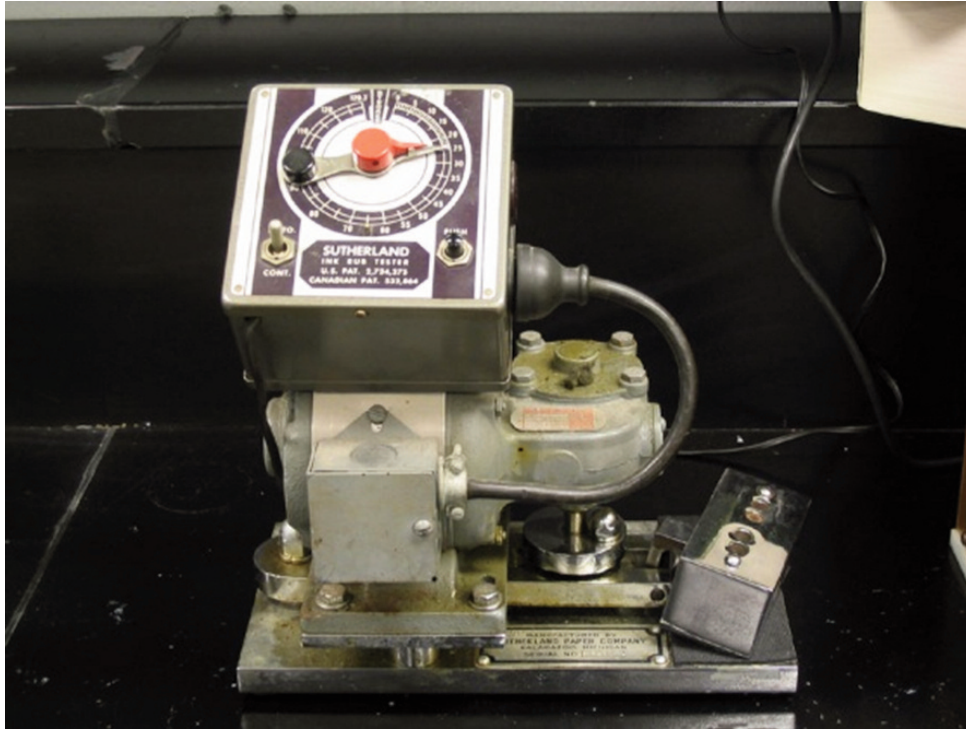
Figure 3. Sutherland Rub Tester used in this study.
