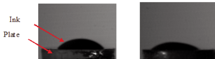
Figure 7: Droplet on water washable plate (left), on conventional plate (right)
