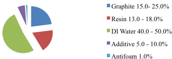
Figure 3: Composition of water based conductive ink
