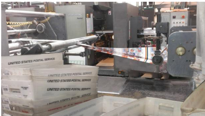
Figure 2: Mail-trays, inline finishing on web press
