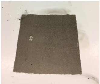
Figure 4. Damaged ink film on cover paper at 2600 μs pulselength
