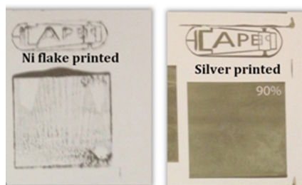
Figure 2. Print results of the optimized Ni ink (left) and flexo silver ink (right)
