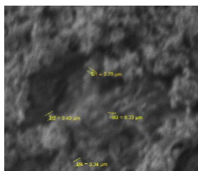
Fig 1. (h) SEM images of 60 weight % of \text{TiO}_2 nanoparticles coated paperboard sample.
