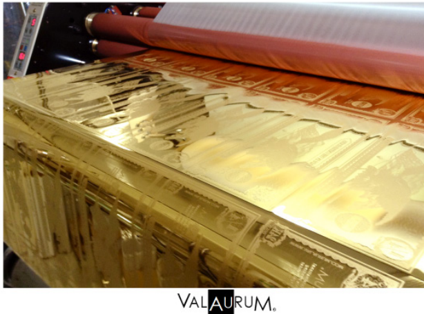
Figure 3. Rolls of Aurum coming out of the gold coating process
