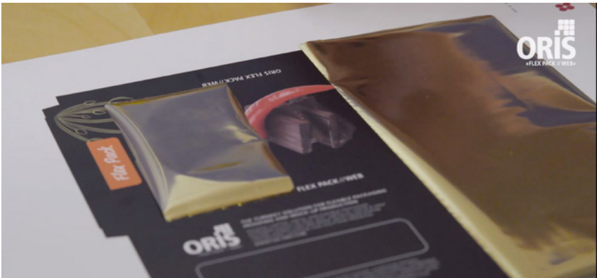
Figure 18 – Positioning of Cold Foil over adhesive area for application
