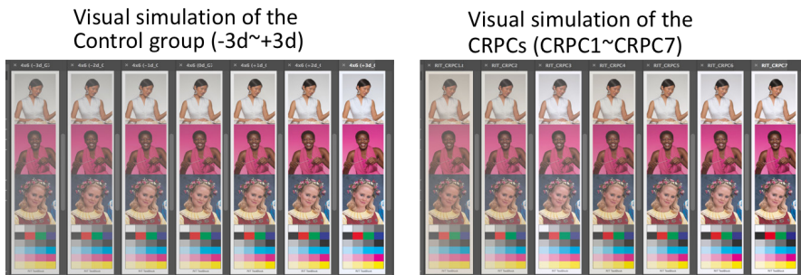
Figure 18. Visual simulation of the RIT test block images using 7 control group datasets and 7 CRPC datasets. With the equal 95 th percentile \Delta E_{00} of 3 between adjacent datasets in the control group, the group of images appear more consistent compared to the CRPCs-based images.
