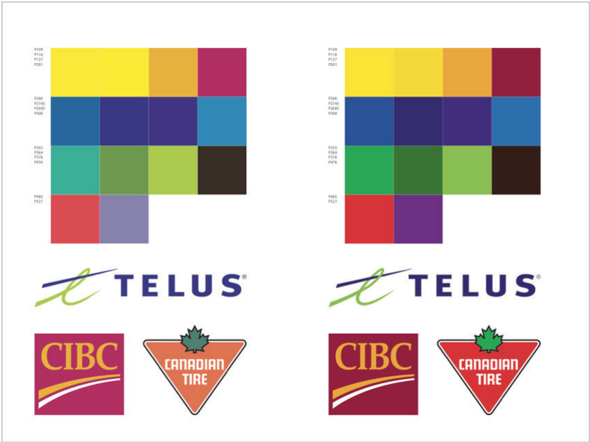
Figure 3: Test chart to test the Pantone color used in this study. The left side of the chart is the expanded gamut version and the right side is the four-color process version of the same Pantone colors.
