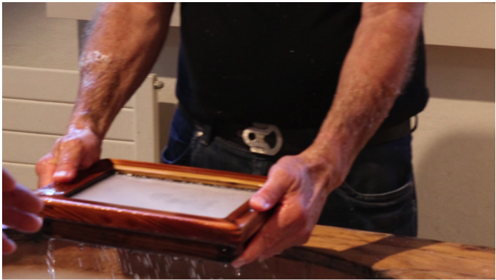
Figure 5: Vatman filling the mold with pulp solution
