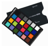
Figure 11. The target for calibrating Xrite Colorchecker photo systems Source: Color Confidence, 2019.
