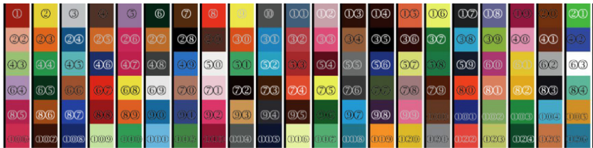
Figure 12. Control strip with 126 patches and identification of each color Color Universe of the strip: colors from all color quadrants
