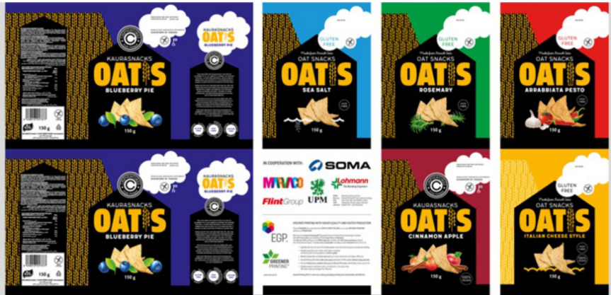
Figure 7: Co-printing of six OATIS designs in a single run with ECG (Image: Marvaco)
