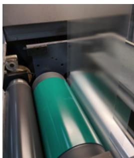
Fig.5 Left: Application of water-based deinking primer on an in-line flexo coater. Right: Slit and sleeved reels ready for deinking testing.
