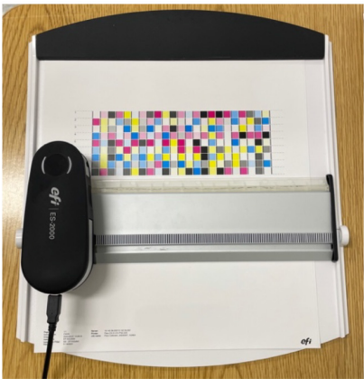
Figure 2: Offline measurement using the EFI ES-2000 spectrophotometer
