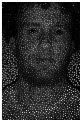
Fig. 6: Projected dots during the unlocking of an iPhone (ardo111 2017)
