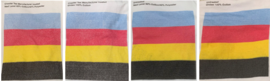
Figure 9. CheaterTee and untreated fabrics following laundering five. CheaterTee on the left and untreated on the right.
