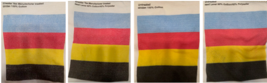
Figure 8. CheaterTee and untreated fabrics following laundering one. CheaterTee on the left and untreated on the right.
