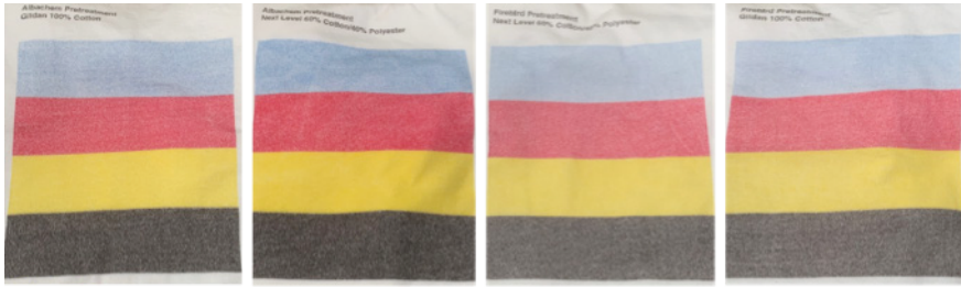
Figure 7. AlbaChem and Firebird fabrics following laundering five. AlbaChem samples are on the left, and Firebird on the right.
