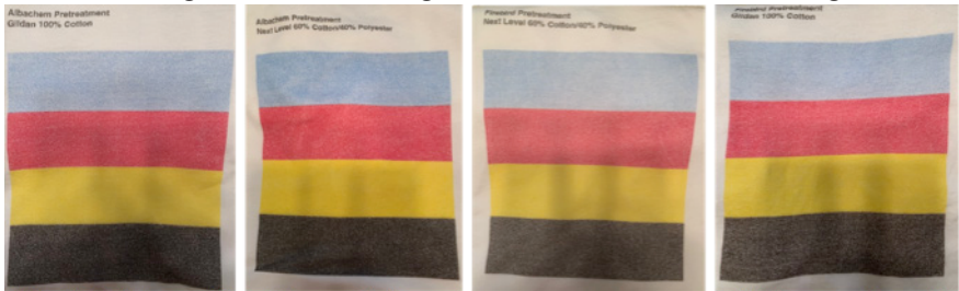
Figure 6. AlbaChem and Firebird fabrics following laundering one. AlbaChem samples are on the left, and Firebird on the right.
