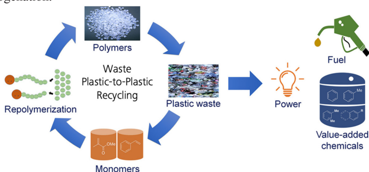
Fig.6: Thermochemical Recycling of Waste Plastics by Pyrolysis (ACS Publications – American Chemical Society 2022)
