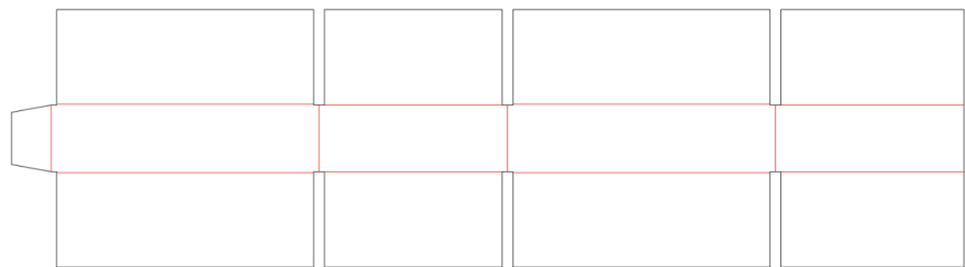
Figure A1: The standard RSC dieline used in testing.
